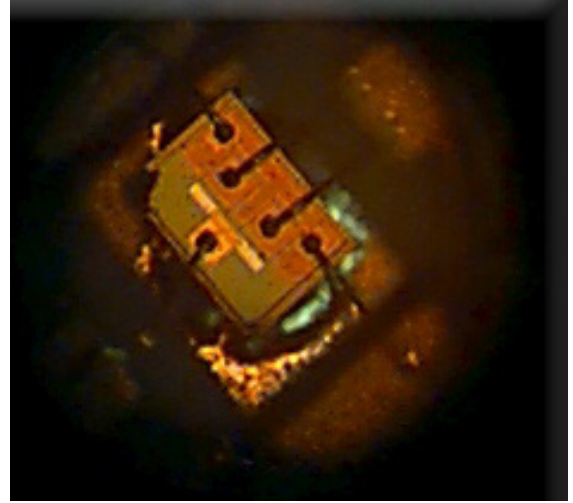
Figure 3. MESFET transistor mounted through circuit substrate for optical biasing.
